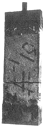
Fig. 2. Uniaxial tension test specimen after rupture
