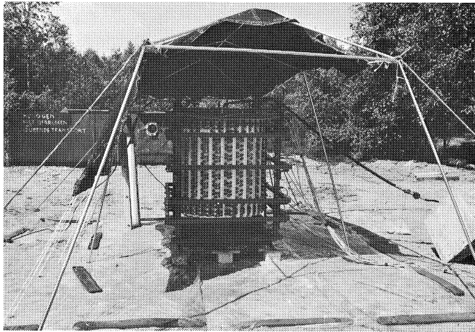
Fig. 20. Model pressure vessel before being loaded by internal gas pressure
