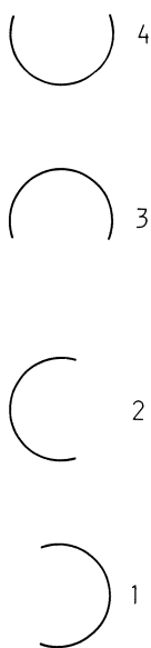
Fig. 4. Location of horizontal tendon layers in relation to one another.
