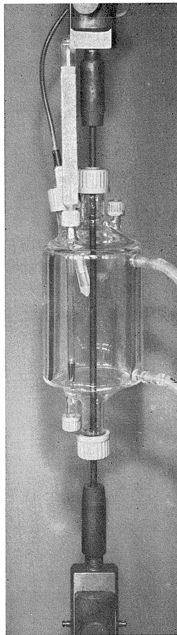
Fig. D5. Double-walled corrosion cell, used in the standardized endurance tests in 20% \text{NH}_4\text{NCS} . The thermometer and calomel cell are visible.
