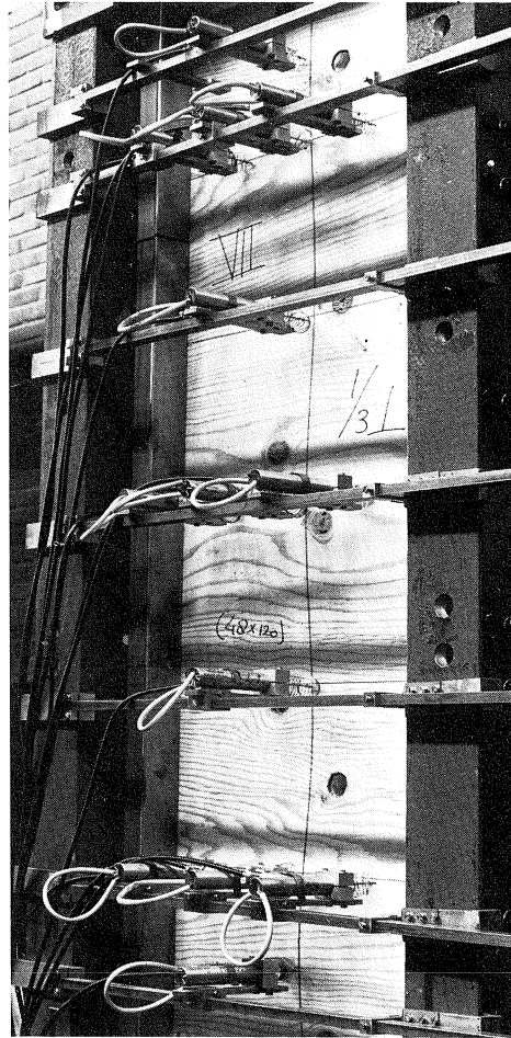
Test specimen with clamped vertical edges. Face veneer horizontal, i.e., perpendicular to the direction of the load. \alpha = 3 ; 4 halfwaves.
