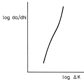
Fig. 14. Crack growth rate ( da/dN ) as a function of the stress intensity factor range ( \Delta K ).
