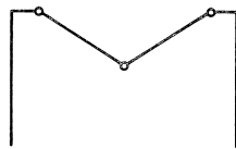
Fig. 3. Collapse mechanism when M_k > M_{pb} .
