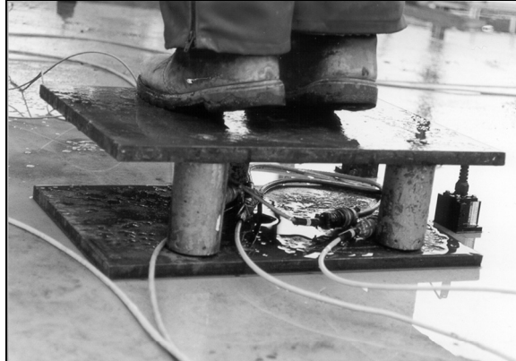
Figure 2: Load source heel drop, measured with load cells
