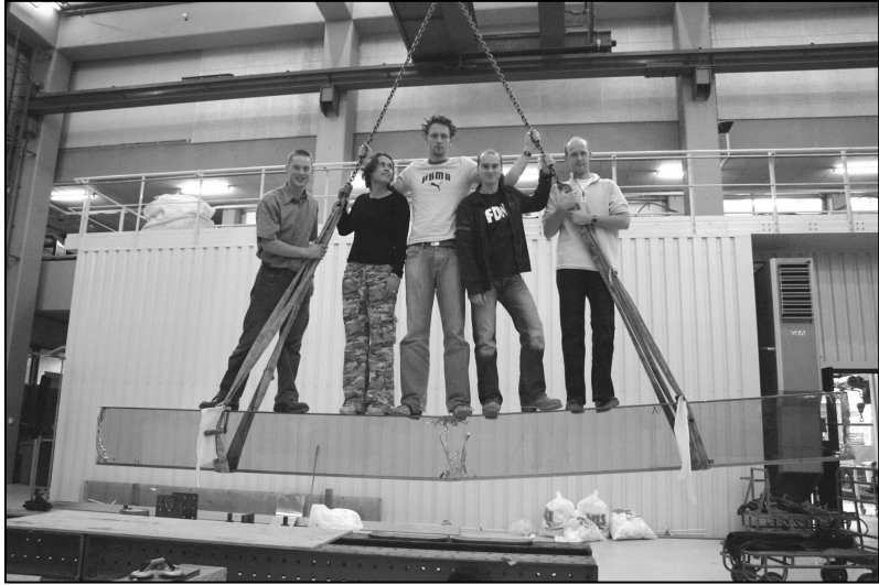
Reinforced glass component with post-peak residual strength; The beam is loaded by TU Delft students and faculty members.
