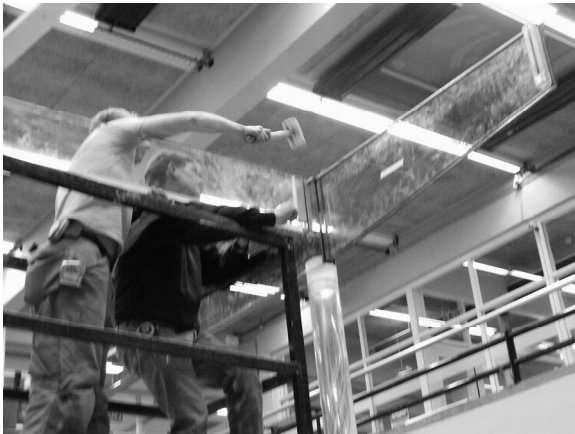
Figure 2: Low cycle impact loading of the joints
