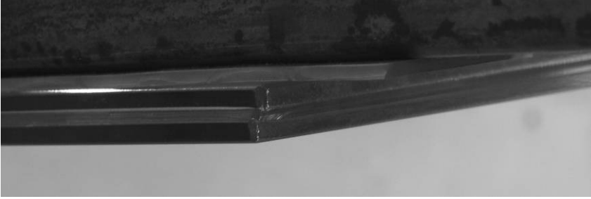
Figure 14: Relative shift of glass plates during the bending process of PVB.4 laminates
