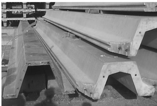
Figure 18: Prestressed sheet piles cast with SCFRC (left: C90/105) and conventional concrete (right: B55/67 concrete with additional bar reinforcement)
