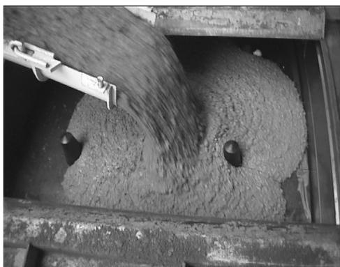
*Figure 22: Orientation of the pipe during casting and distribution pattern of SCFRC*
