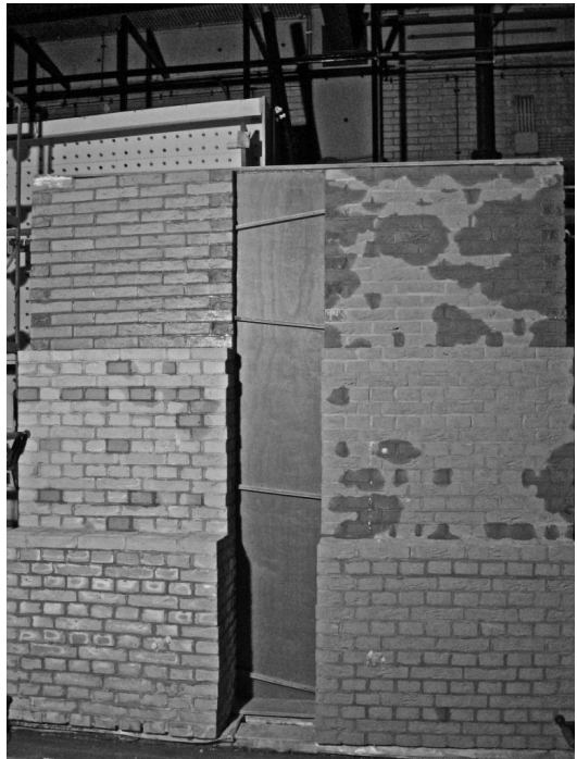
Figure 1. Leakage in test masonry walls
