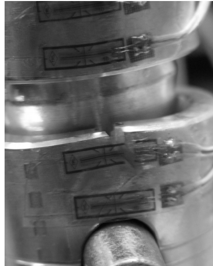
Figure 13. Structural failure due to extended cracking at the centre point
