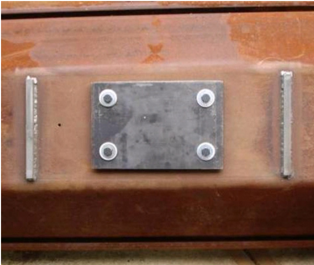
Figure 5. Coupon sensor under construction
