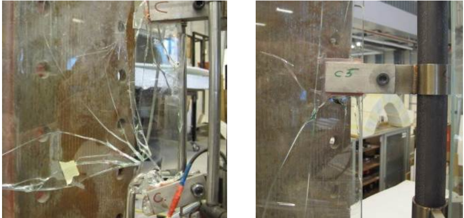
Figure 12: Locally failed glass pane in test 3
