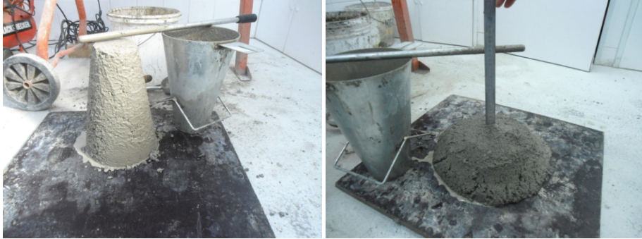
Figure 4: PU-based concretes optimized for blocks (left) and panels (right)
