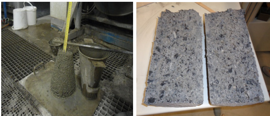
Figure 6: Slump test on tyre rubber based concrete (left) and aggregates distribution observed in the cross section (right)
