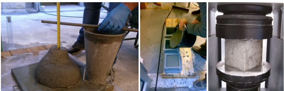
Figure 3: Slump evaluation and preparations of cubic specimens for compressive testing (from left to right)
