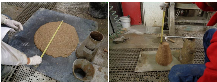
Figure 1: Example of workability for cyclone / \mu -silica with PU aggregates: 580 mm slump flow (after 4 min) and 100 mm slump (after 30 min)
