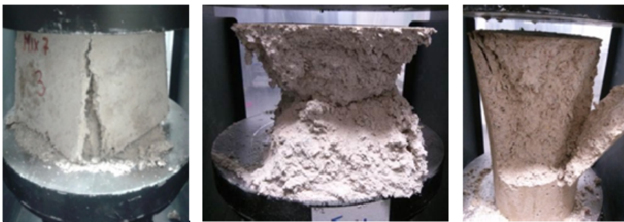
Figure 2: Disintegration of the specimen during the compression strength test showing that the interior of the specimens did not harden
