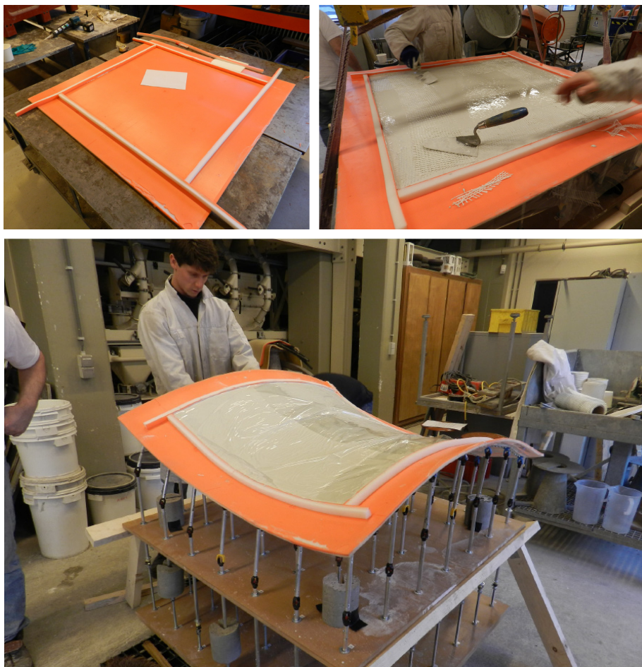
Figure 14: Process of edge positioning, casting and deformation
