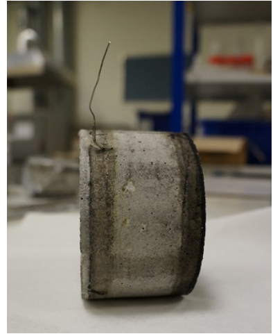
Figure 1: Specimen with embedded titanium mesh. The wire coming out of the specimen on the left is from the embedded mesh.
