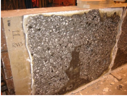
Figure 1: Spalling damage, as observed after full-scale fire testing, can be limited to the surface of the concrete slab (left) (Jansson & Boström, 2008) or in the most severe case considerably reduce the structural capacity, as shown for a loaded tunnel lining segment (right) (Dehn, et al., 2010)
