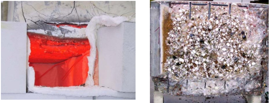
Figure 11: Cracking of a HSC slab during thermal exposure according to the RWS fire curve (left) and resulting spalling damage (right) (Horvath, et al., 2004)
