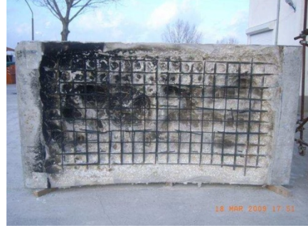
Figure 1: Spalling damage, as observed after full-scale fire testing, can be limited to the surface of the concrete slab (left) (Jansson & Boström, 2008) or in the most severe case considerably reduce the structural capacity, as shown for a loaded tunnel lining segment (right) (Dehn, et al., 2010)
