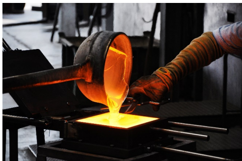
Figure 1: Casting glass at Poesia
