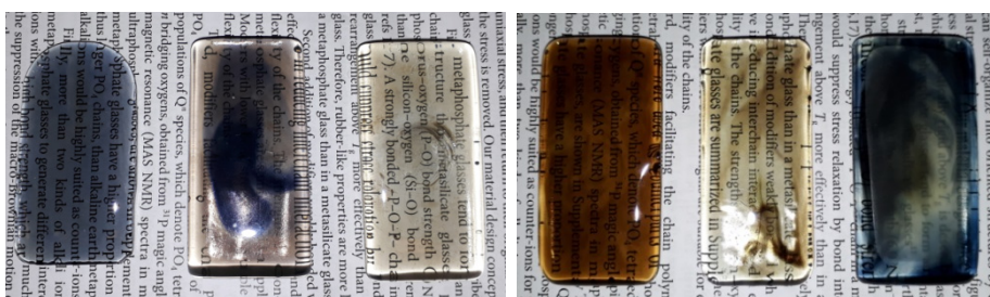
Figure 6: Samples consisting of 12.5% slag melted at different temperatures: 1150^\circ C , 1250^\circ C , and 1350^\circ C , respectively
