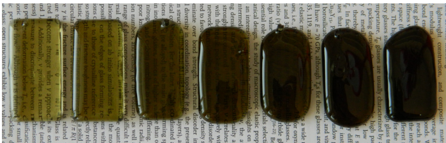
Figure 8: The samples containing fly ash. From the left to the right: 75\text{KPO}_3\text{-}12.5\text{FA}\text{-}12.5\text{Al}_2\text{O}_3 , 70\text{KPO}_3\text{-}15\text{FA}\text{-}15\text{Al}_2\text{O}_3 , 65\text{KPO}_3\text{-}20\text{FA}\text{-}15\text{Al}_2\text{O}_3 , 60\text{KPO}_3\text{-}20\text{FA}\text{-}20\text{Al}_2\text{O}_3 , 60\text{KPO}_3\text{-}25\text{FA}\text{-}15\text{Al}_2\text{O}_3 , 60\text{KPO}_3\text{-}30\text{FA}\text{-}10\text{Al}_2\text{O}_3 , 55\text{KPO}_3\text{-}35\text{FA}\text{-}10\text{Al}_2\text{O}_3
