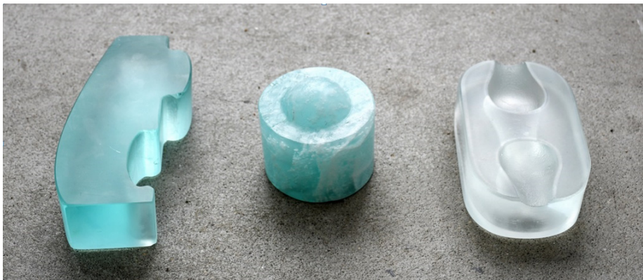
Figure 17: PPG furnace waste aquamarine cast at 1120°C (left) and at 860°C (middle). PPG Starphire cast at 1120°C (right)
