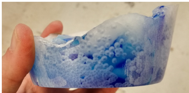
Figure 13: Glass sample from the flowerpot used during the 860°C casting experiment, showing the formation of crystals
