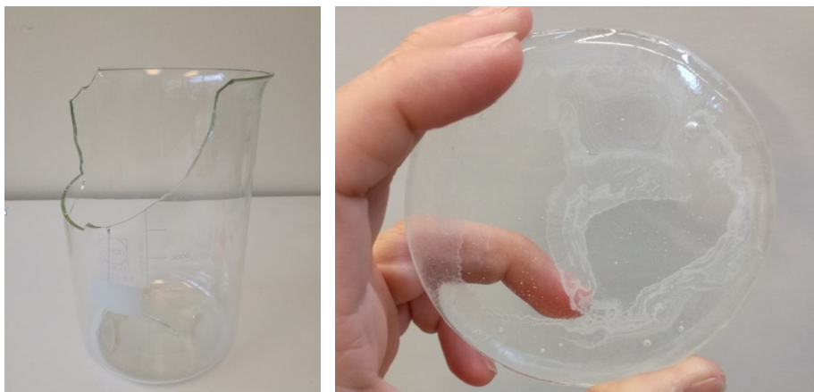
Figure 27: Borosilicate labtube before and after casting at 1200°C
