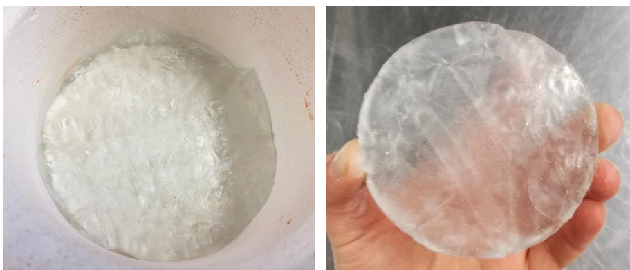
Figure 20: Czech glass cast at 950°C. Post-processing is required to remove the shrinkage of the top surface and reveal the actual transparent glass.
