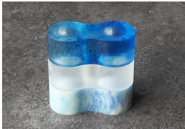
Figure 11: Glass samples cast employing Sprucepine clear and blue glass waste (top and bottom) and lead crystal (middle element). The figure shows the effect of casting temperature to the structure of the glass component. Although the top and bottom sample are cast using the same glass, the one below, cast at 860°C crystallized, in comparison to the clear blue component on top, cast at 950°C.
