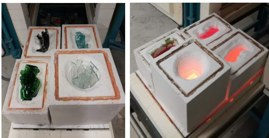
Figure 7: Kiln-casting experiment at 1120^\circ\text{C} , portraying the differences in luminosity among the various coloured samples
