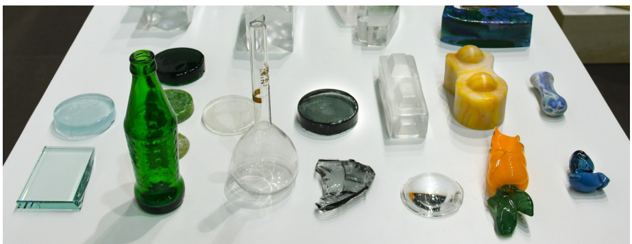
Figure 31: Successful casting of pieces of (from left to right) float glass, bottle, laboratory tube, computer screen panel, lens, and mouth blown glass, demonstrating the numerous possibilities that arise in creating unique building components
