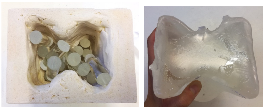
Figure 28: Borosilicate extruded rods successfully re-cast at 1120°C
