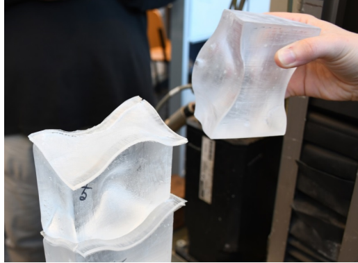
Figure 11: Prototype of a 3 mm thick, cast PU70 interlayer
