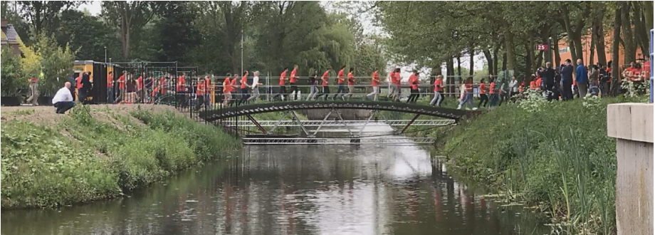
Figure 30: Load case 3, 60 running students, approximately 14.7 kN/m
