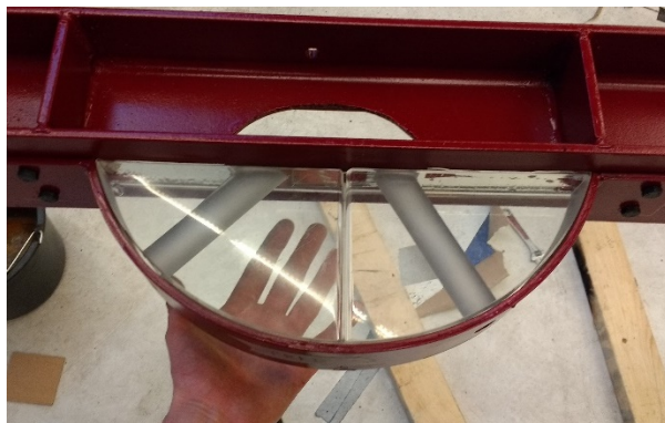
Figure 21: The node after placement in the truss
