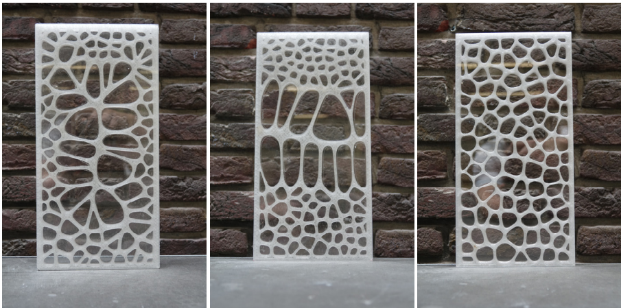
Figure 20: Thin glass panels with 3D-printed PETG Voronoi core patterns [Neeskens, 2018]
