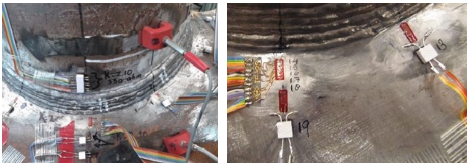
Figure 29: Left: Strain gauges and Manual ACPD current; Right: strain gauges
