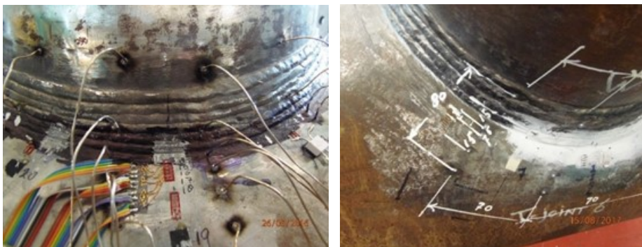
Figure 30: Automated ACPD, reference spacing 15 mm, 1 Amp current
