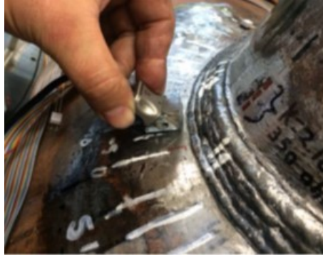
Figure 31: Validation by phased array
