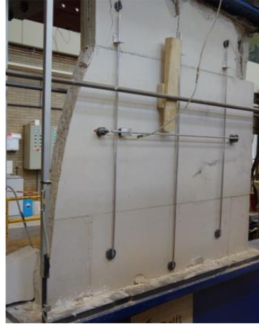
(c) CS element masonry failure mode
