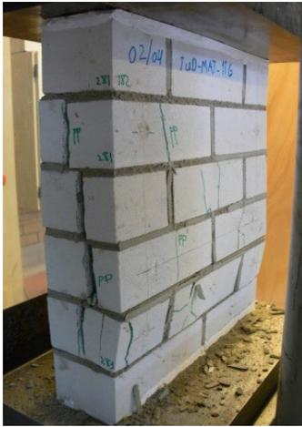
(b) CS brick masonry failure mode
