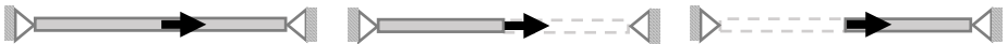
Figure 4. Minimizing the volume of a single rod (complete left) by transforming it into a tensile (middle) or compressive rod (complete right)
