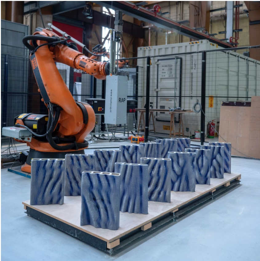
Figure 9. A series of 3d-printed tiles for the New Delft Blue gates using a robotic arm the workshop at Studio RAP, ©Studio RAP
