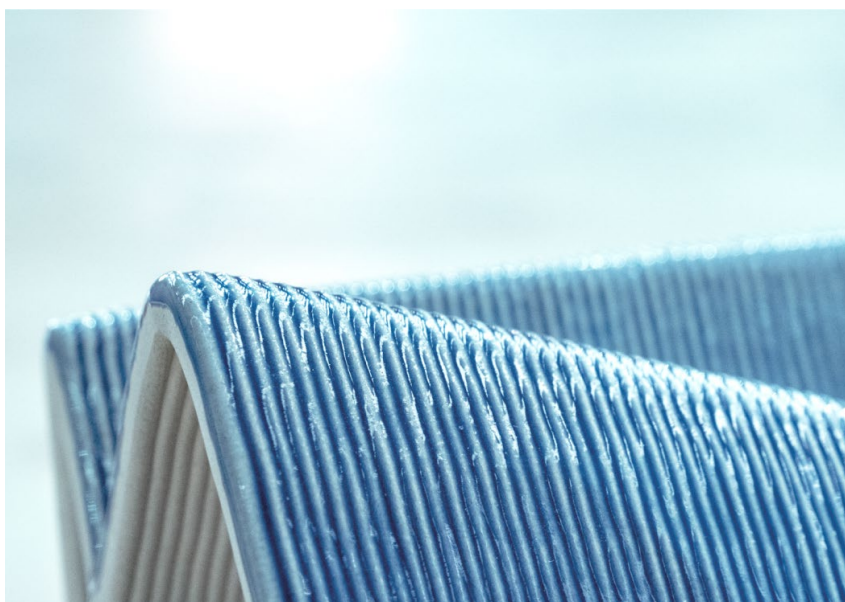
Figure 10. Close up photo of a 3d-printed ceramic tile showing the 3d-printed layers and the transparent blue glaze, ©Studio RAP
