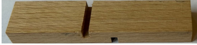
Figure 1a. Standard lap joint specimen (Beech, Adhesive surface l \times w = 10 \times 20 mm, width w adapted per series to the required load level)
